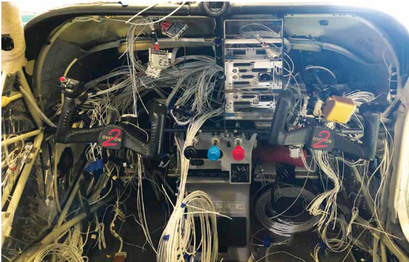
*New avionics add enormous value and capabilities to any aircraft. But it's important that the magnitude of the upgrade is justified by the performance of the airplane and the pilot. This nest of wires is the soon-to-be-new all-glass panel of a Mooney Ovation owned by my friend Tom McPherson. A high-performance plane if there ever was one, I am quite sure Tom will use every ounce of this new technology in the years ahead. Could the same be said about an upgrade to a tired Cessna 152?*
